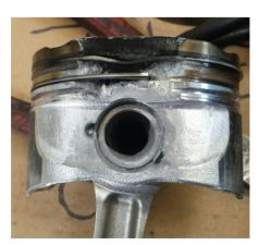
If cylinder walls are not damaged and one or more of the pistons are found fractured, replace all four spark plugs, all four ignition coils (apply dielectric grease to the spark plug boots), the fuel injector of the cylinder(s) that had damaged pistons, all four piston kits, all ring sets for all four pistons, all rod bearings, all four connecting rod assemblies and other components necessary when pistons are replaced.
