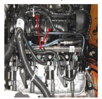
Inspect for a holding clip that secures the engine harness to the fuel line bracket. See Photo Below.
