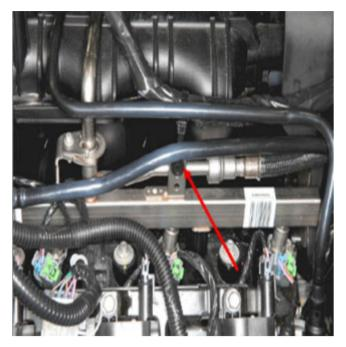
If the holding clip is missing, you will need to get a retaining clip to install.
