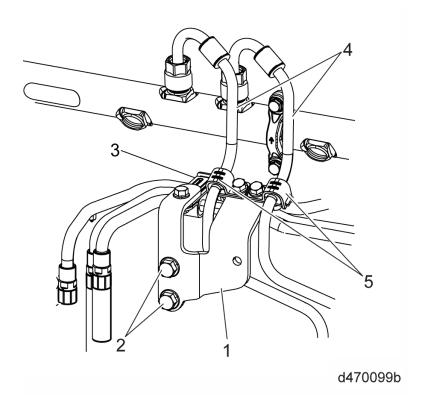
2. Clean the sealing area inside the high pressure fuel pump outlet fittings using a clean lint-free cloth. The photo shown below is of KM59 GEN1 High Pressure Fuel Pump Fittings.
