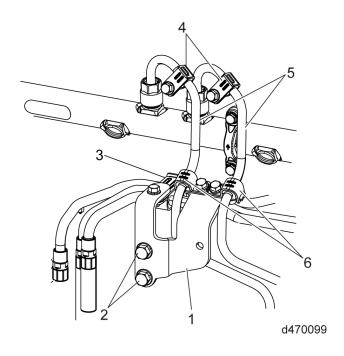
**NOTE:** The graphic below illustrates DD engines with permanent vibration dampers on the high pressure fuel rail feed lines.
