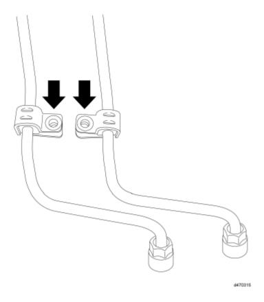
**NOTE:** DO NOT use new high pressure fuel rail feed lines that do not have new vibration dampers installed.
