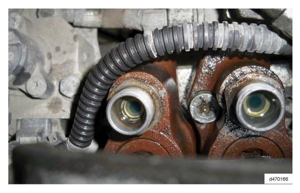
3. Clean the sealing area inside the high pressure fuel rail using a clean lint-free cloth. The photo shown below is of KM59 GEN1 high pressure fuel rail fittings.
