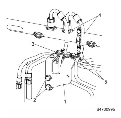
**NOTE:** New P-clips (2) <u>MUST</u> be installed perpendicular to the bracket (1) and parallel with each other. Hold P-clips in place during tightening to avoid rotation of the P-Clips; see graphic below.
