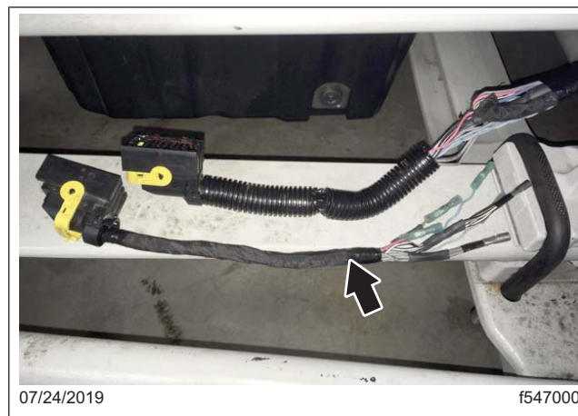
Fig. 5, MCM 21-Pin Jumper Harness with Pre-Installed Splices
