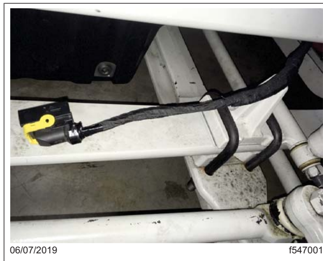
Fig. 6, Wrapping the Harness with Fiber Tape
