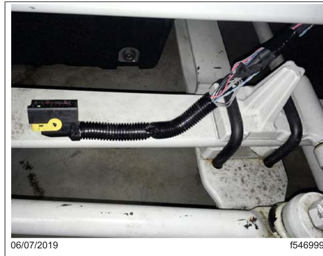
Fig. 4, Separating the Wiring to Identify the Circuits
