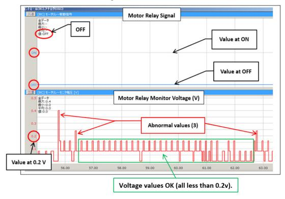
**Step 3:** If either **Scenario 1** or **2** described above is confirmed, the VDCCM&HCU must be replaced.
