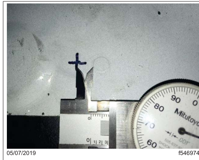
Fig. 5, Measuring Between the Floor Mound and the Rivet
