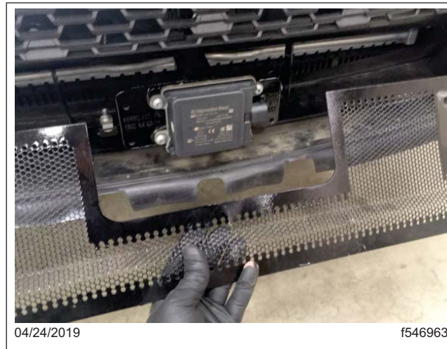
Fig. 3, Rock Guard Installation
