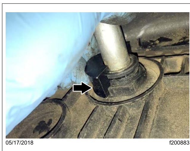
Fig. 6, Half of Collar Assembly Installed
