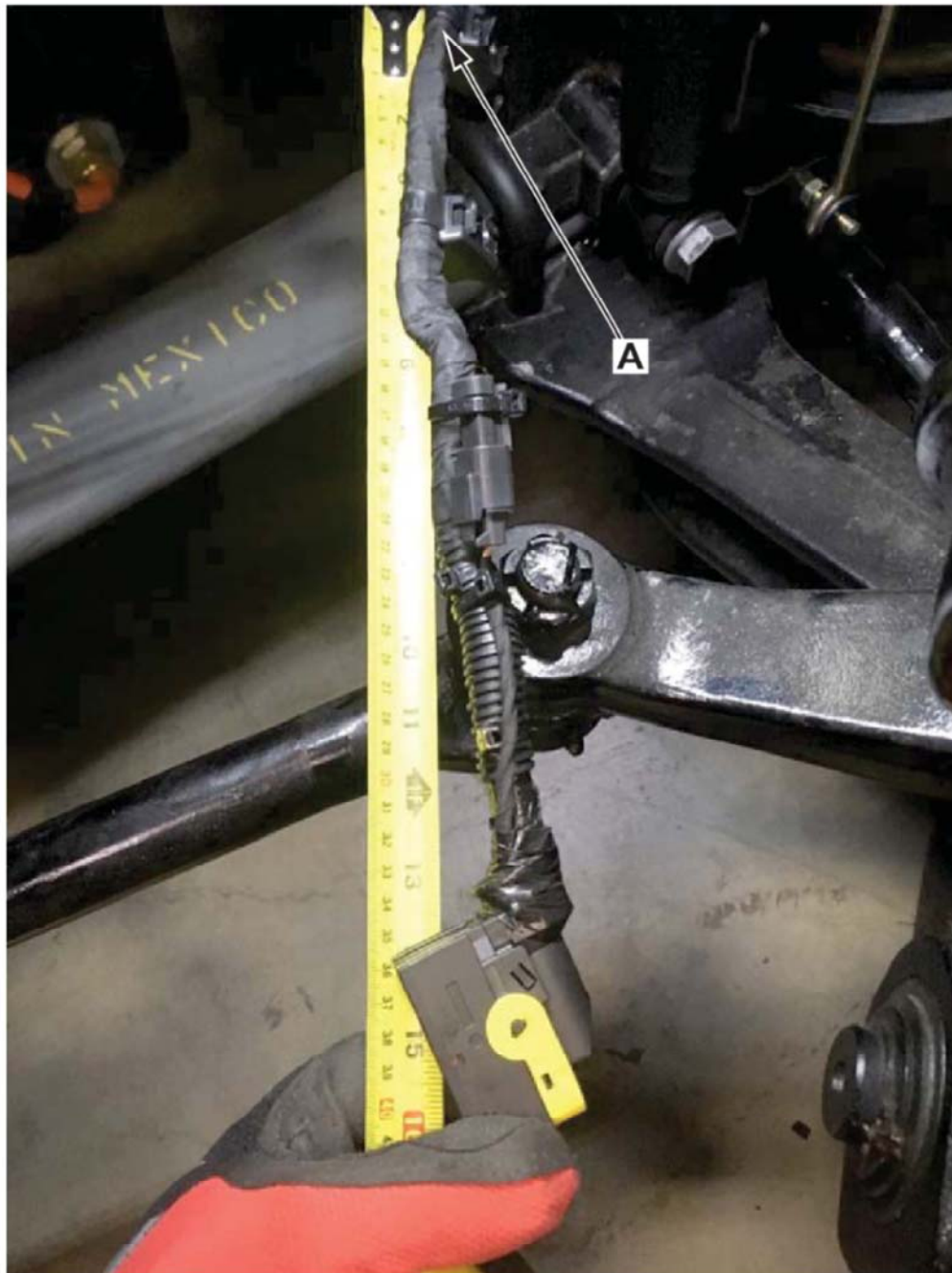
Fig. 1, Splicing Point on the MCM 21 Pin Jumper Harness
