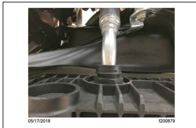
Fig. 2, Cooler Line Connection with Original Plastic Cap and Spring Clip
