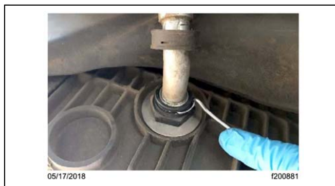
Fig. 5, Removing the Spring Clip
