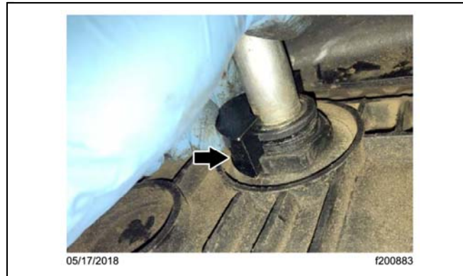
Fig. 6, Half of Collar Assembly Installed
