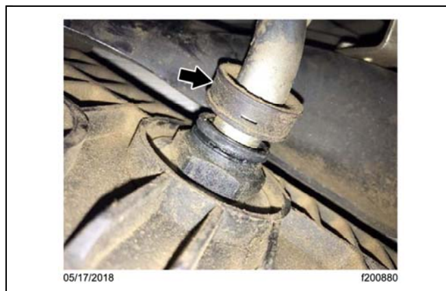
Fig. 4, Removing the Plastic Cap
