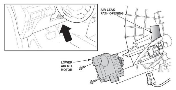
7. Mark the gear on the motor and the gear on the vehicle. This will help with alignment during installation.
