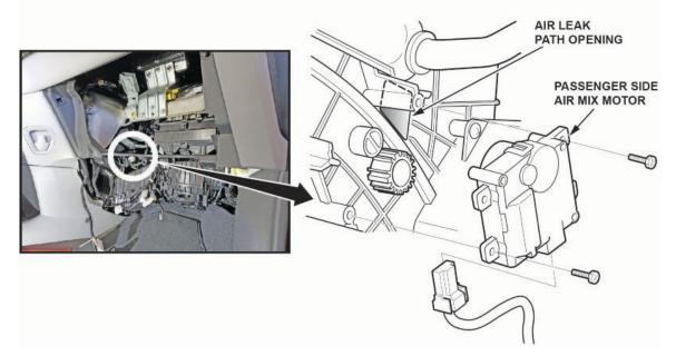
22. Mark the gear on the air mix motor and the gear on the vehicle. This will help with alignment during installation.
