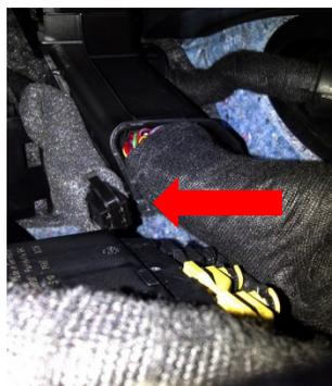
4 pin connector is wrapped in foam near the vehicle electrical module.
