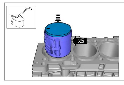
Note! Make sure that the direction arrow points towards the front of the engine.
