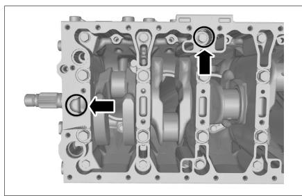
Caution! Make sure that the gaskets are correctly located.
