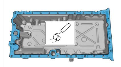
Note! The component must be installed within 5 minutes of applying the sealant.
