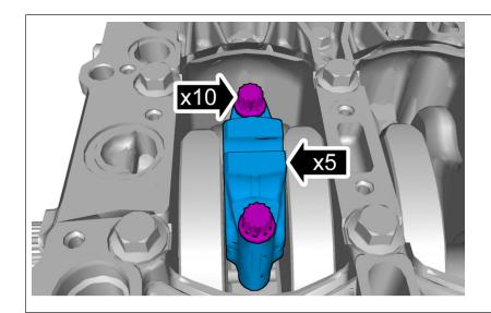
Caution! Note the position of the bearing caps in relation to the rotation of the crankshaft. The bearing caps are not interchangeable.
