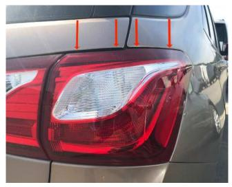
If you encounter a vehicle with the above concern, measure the gap between the tail lamp and the body side, at the locations shown in the picture above, and contact the engineer below with your findings.
