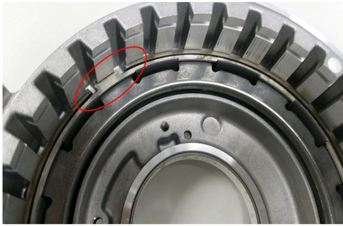
**Important:** During assembly, position the 1-3 clutch return spring ring as shown in the attached picture to aid in retainer installation.
