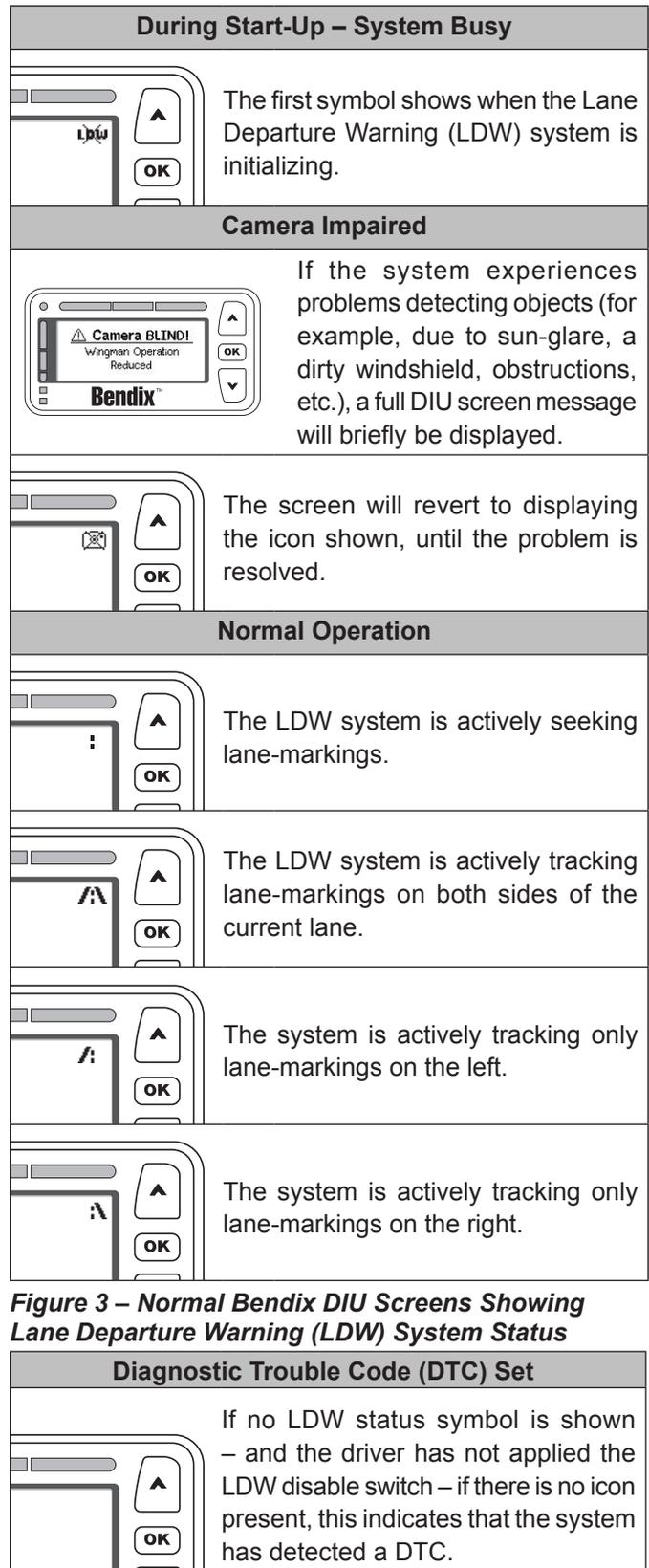
**Figure 3 – Normal Bendix DIU Screens Showing Lane Departure Warning (LDW) System Status**
