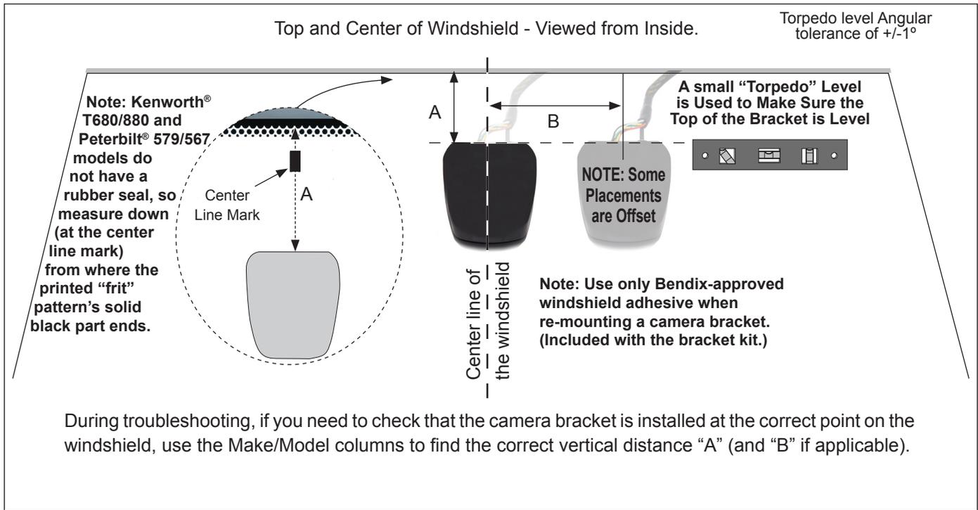
Center the Top of the Bendix™ AutoVue® FLC-20™ camera at the location specified in this table
