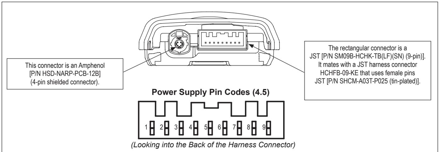
**Figure 9 – Camera and Harness Connector Views**
