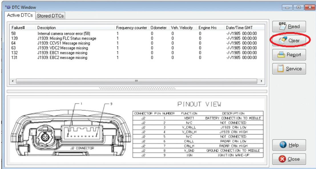
**Figure 10 – Clear Diagnostic Trouble Codes (DTC[s]) Button**
