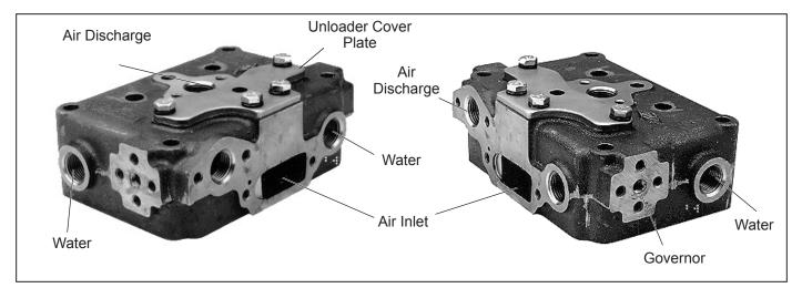
Figure 2 – Cylinder Head
