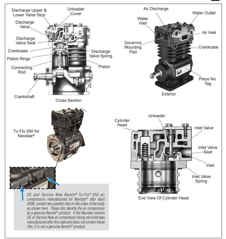
Figure 1 – Bendix® Tu-Flo® 550 Air Compressor
