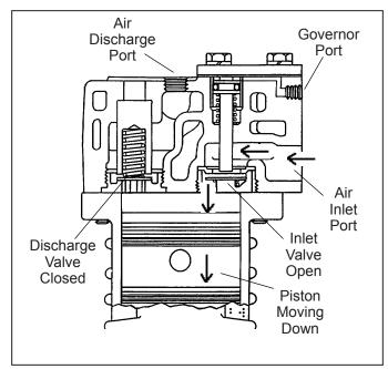
Figure 5 – Operational-Loaded (Intake)
