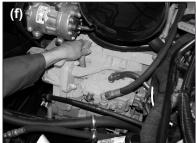
Testing the temperature at the discharge fitting.
