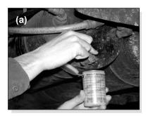
Drain <u>all</u> air tanks (reservoirs) into the Bendix BASIC test cup. (Bendix kit P/N 5013711).
