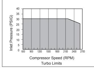
Figure 12 – Turbo Limits Curve
