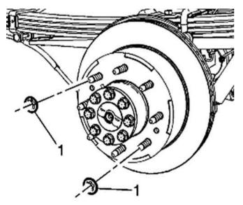
Prior to installing affected Accessory wheels, the dealer technician must remove and discard the tinnerman push nuts (1). Failure to do so may result in unintended lug nut and wheel loosening.
