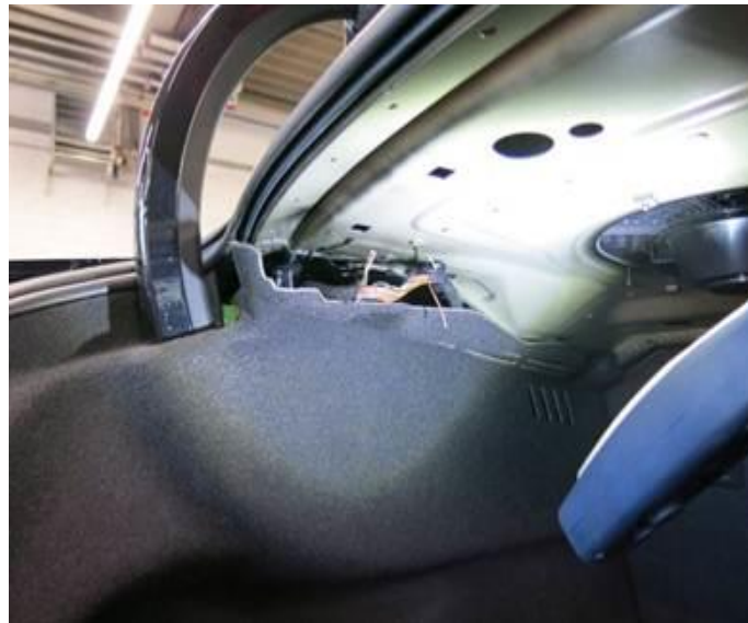
Figure 2. Wire damage at the trunk hinge.
