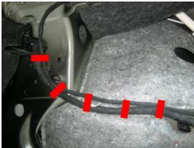
Figure 11. Wrap the wiring harness with textile adhesive tapes at red marks.
