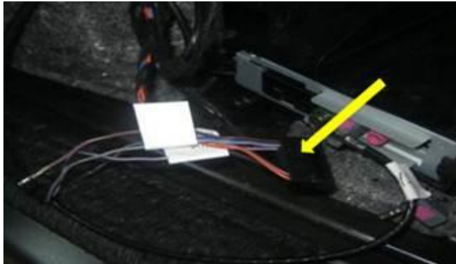
Figure 10. To unlock the contacts, position VAS 1978/29 on the side.
