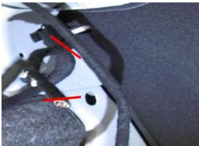
Figure 14. Open the winding of the cut-off vehicle wiring harness to the junction of the main harness on the separable area (red marks).
