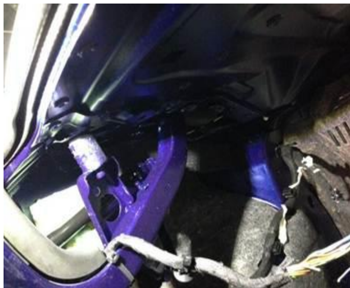
Figure 3. Incorrect wire routing at the trunk hinge.
