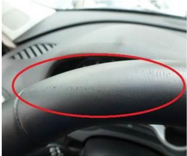
*Figure 2. Example of damage from external impact.*
