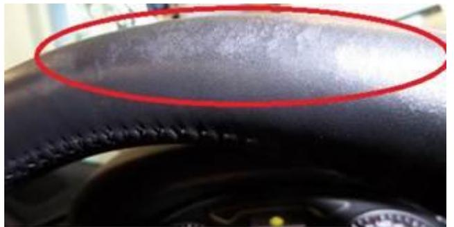
*Figure 3. Example of damage from external impact.*
