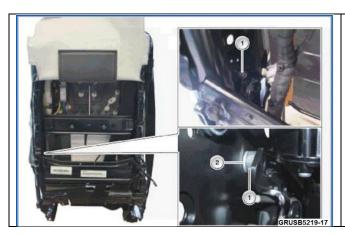
Install (2) washer 07 11 9 904 204 between the limit position (1) and the backrest.
