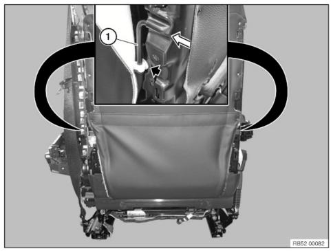
Unclip soft-top bow (1) on left and right and detach from backrest frame.
