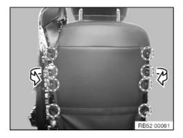
Detach backrest cover on left and right from metal retainer.
