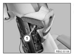
Release screws (1) on left and right.
