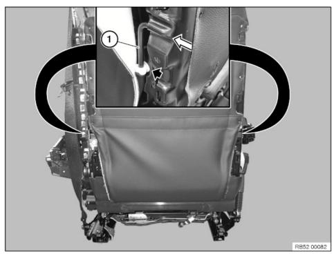
Unclip soft-top bow (1) on left and right and detach from backrest frame.
