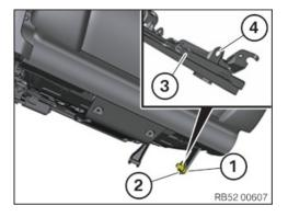
Insert bolt (1) with greased plastic washer (2).
