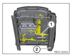
Unclip wiring harness (1) from seat rail (2).
