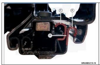
2. In addition to the lubrication points indicated in the Repair Instructions, apply lubricating grease (3) **BETWEEN** the reinforcement plate (1) and the outer shell (2).
