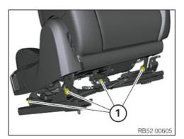
Counter support bolts (1) (do not turn) and remove nuts.
