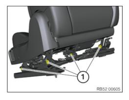
Counter support bolts (1) (do not turn) and tighten nuts.
