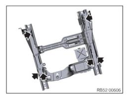
Coat marked contact surfaces with lubricating grease, Klübersynth LF 44-22 (part number 83 23 0 396 713).
