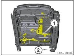
Clip wiring harness (1) into seat rail (2).
