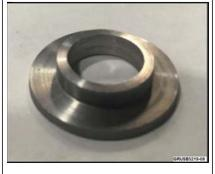
As of March 2019 production, two machined washers (shown) were added to the bottom of the inner seat rail on the driver's side (left rear) of the 60/40 split 2nd row seat.
