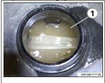
Coolant in the low temp cooling circuit may also have an acrid smell and discoloration (1).
