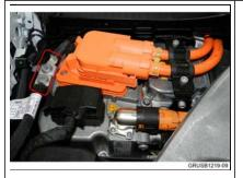
Remove both grounding cables at the EME
