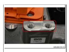
2. Clean the contact surface of both grounding cables and the ground support point at the EME using 1200 grit emery cloth or equivalent to remove any corrosion or oxidation.
