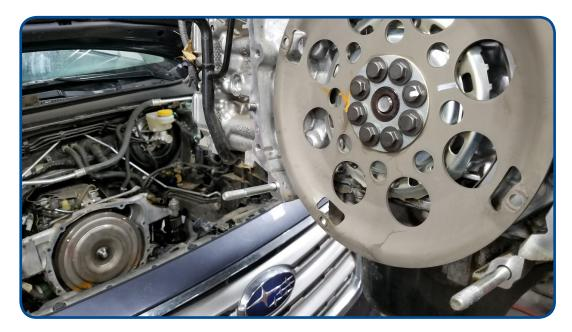
The photo above shows the nose of the torque converter is broken off and remaining in the crankshaft. Also note, there is no torque converter holder tool installed to the transmission.
