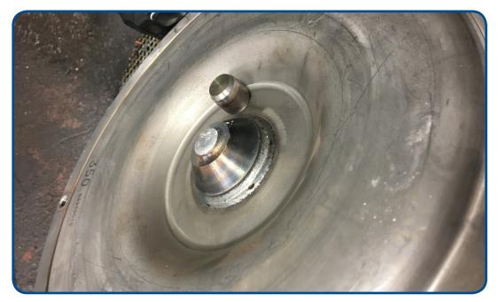
Torque converter with broken nose.
