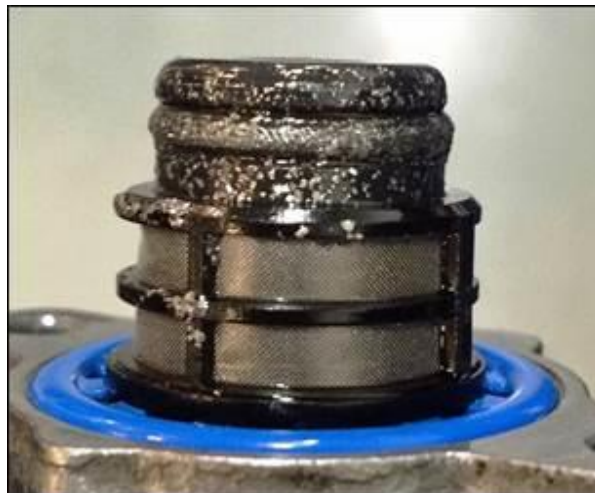
Figure 3. Example of a clear picture showing the metallic particles in the N290 fuel metering valve.
