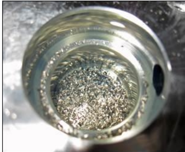
Figure 4. Example of a clear picture showing the metallic particles in the valve bore.
