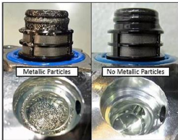
Figure 2. N290 Fuel Metering Valve and Valve Bore
