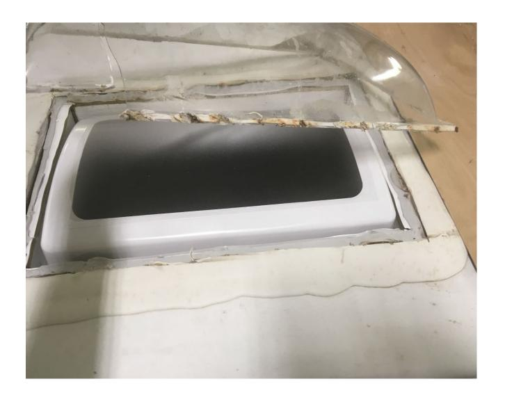
Clean the top side of the inner dome with compressed air and a dry rag to remove any plastic dust.
