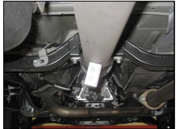
Figure 12. INCORRECT Placement of Digital Angle Gauge
