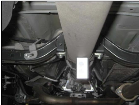
Figure 11. CORRECT Placement of Digital Angle Gauge
