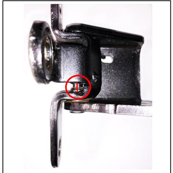
3. Watch the scribe lines while manually moving the slide door forward and backward until just BEFORE the closed position and when the center hinge pivots.
