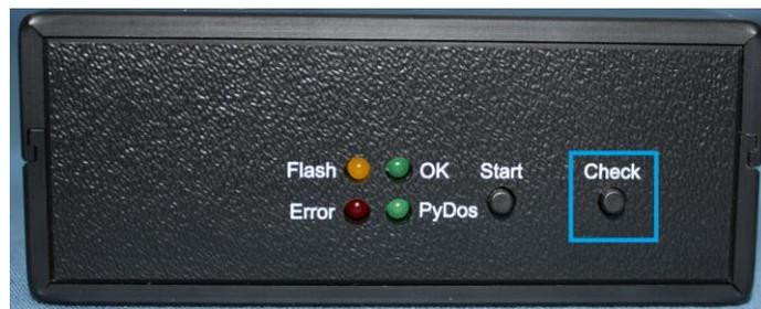
This operation is optional and takes up to 95 s. During this check operation the OK-LED and the Error-LED are flashing alternately.
