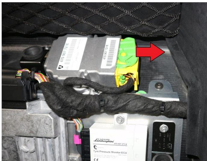
14. Connect the service tool 61653001466 to the Pydos control unit.
