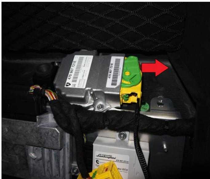
20. Connect the wirings of the Pydos control unit.
