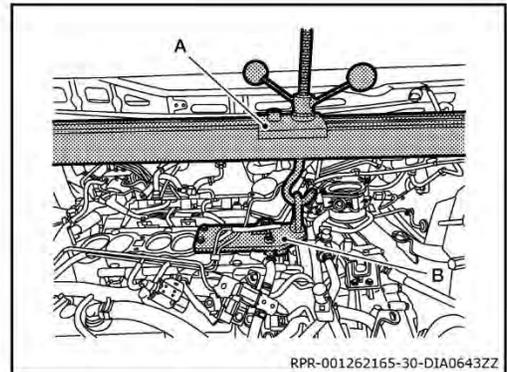
29. Using bubble level (B) on Tool (A) level Tool as shown. Refer to Engine Support Tool Operating Instructions.
