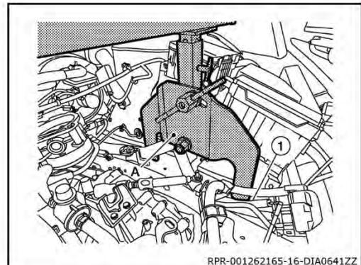
27. Install Tool (A) on top of engine mounting insulator [RH (1)] as shown. Refer to Engine Support Tool Operating Instructions.
