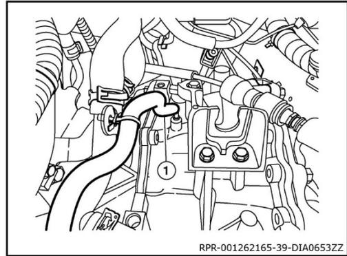
20. Remove bolt (A) from upper torque rod.
