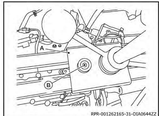
30. Remove nut from engine mounting insulator (front). Refer to Engine Assembly "Exploded View" in the Engine Mechanical section of the ESM.
