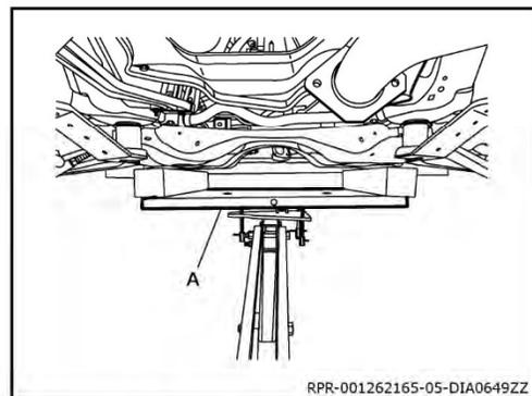
67. Remove front suspension member bolts and front suspension member stays. Refer to Front Suspension Member "Exploded View" in the Front Suspension section of the ESM.
