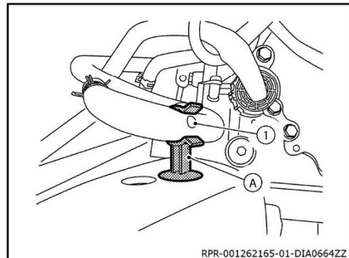
65. Remove rear torque rod bolt. Refer to Engine Assembly "Exploded View" in the Engine Mechanical section of the ESM.
