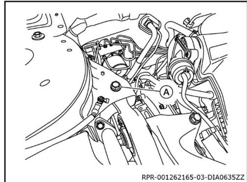
21. Remove fuel tube bolts (A).
