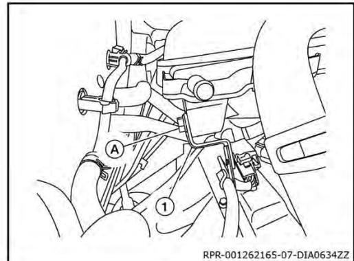
18. Loosen the intake manifold collector bolts and nuts in reverse of the sequence shown, then remove the intake manifold collector and gasket.
