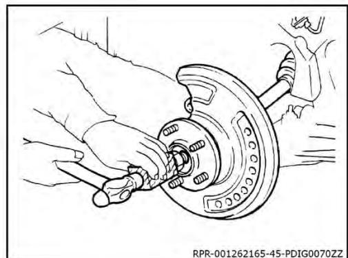
42. Remove the wheel hub lock nut (LH/RH).
