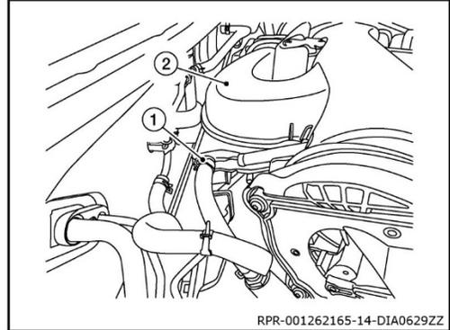
8. Remove bolts (A) and set VIAS control solenoid valves (1) aside.
