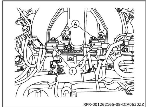
9. Disconnect vacuum hoses (1) from intake manifold collector (2).
