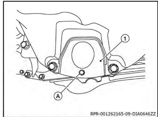
58. Remove torque converter nuts. Refer to Transmission Assembly "Exploded View" in the Transaxle and Transmission section of the ESM.
