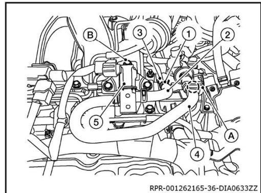
13. Release pawl and remove hose (4) from retainer (A).
