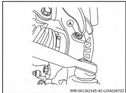
37. Remove and discard cotter pin from front drive shaft (LH/RH).
