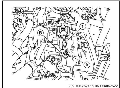
5. Disconnect the harness connector (A) from the transmission range switch (1).
