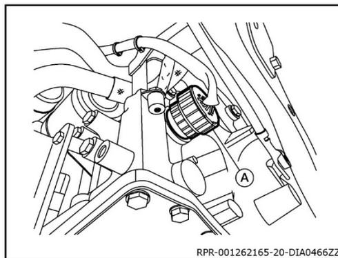
76. Disconnect the harness connector from the output speed sensor. Refer to Output Speed Sensor "Exploded View" in the Transaxle and Transmission section of the ESM.
