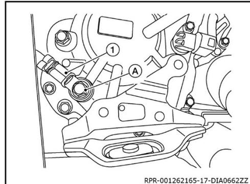
64. Remove water hose (1) from retainer (A).
