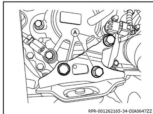
63. Remove bolt (A) and position ground (1) aside.
