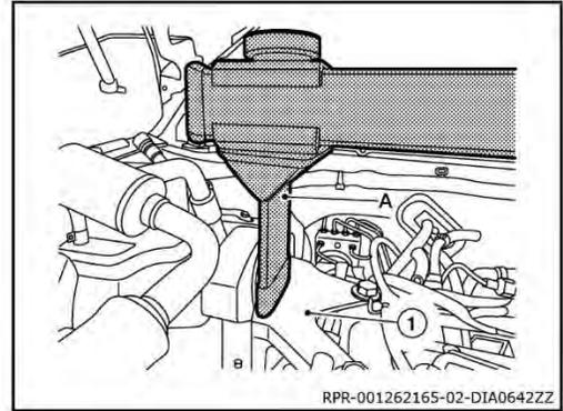
28. Install Tool (A) to Tool (B). Refer to Engine Support Tool Operating Instructions.
