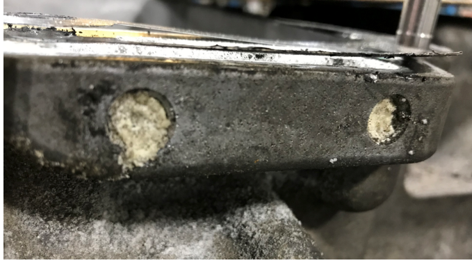
Clogged vent ports
