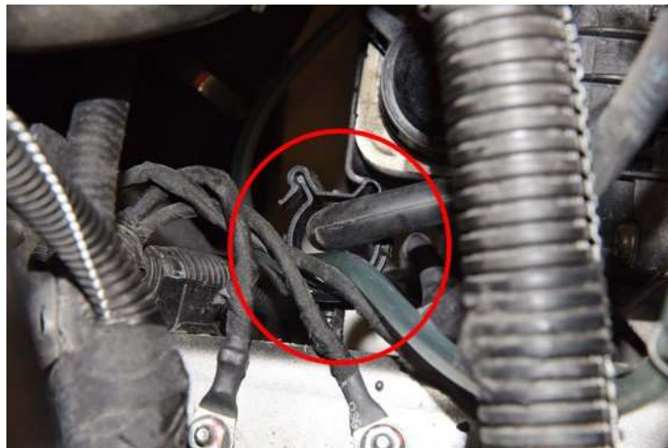
Fig. 14 Clamp Installed On Support
