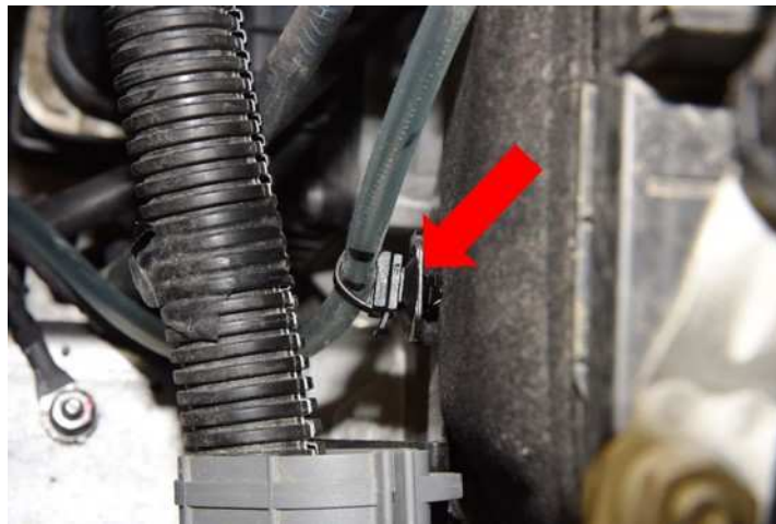
Fig. 12 Clamp Installed On Bracket
