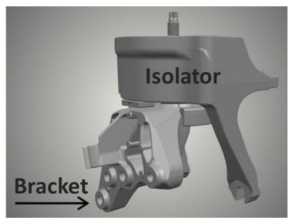
Replace the bracket on any ProMaster with a VIN built before 10/23/2015.
