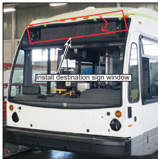
Figure 35 - Install Destination Sign Window
