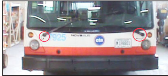
Figure 48 - Install the Windshield Wipers
