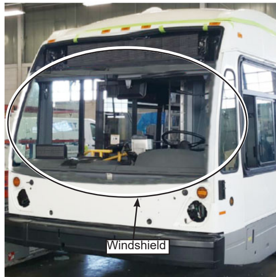
Figure 16 - Remove the Windshield
