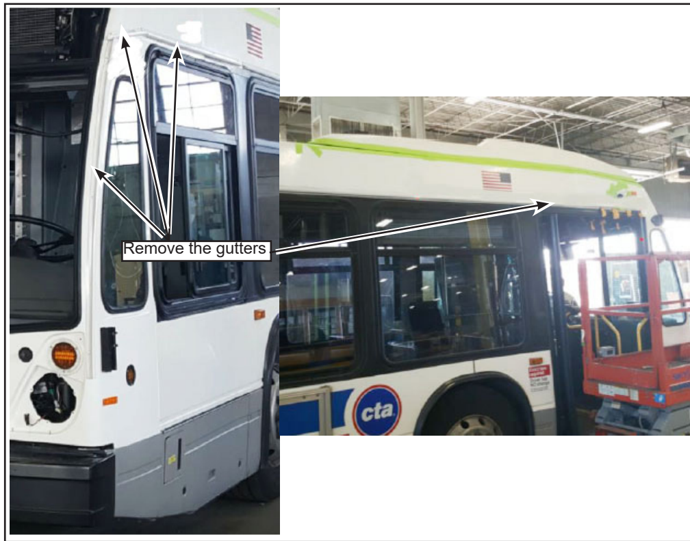
Figure 10 - Remove the Gutters
