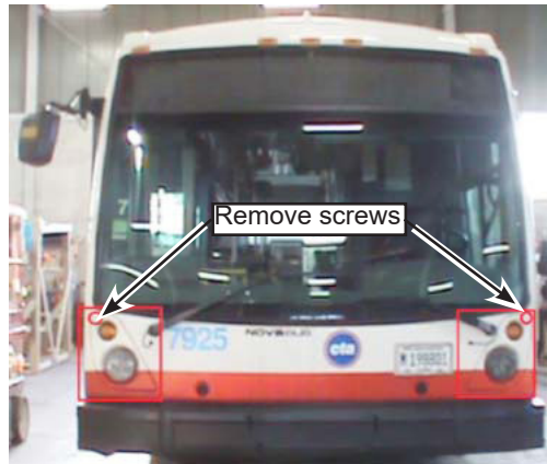
Figure 4 - Remove the Bezel, Turn Signals and Headlights
