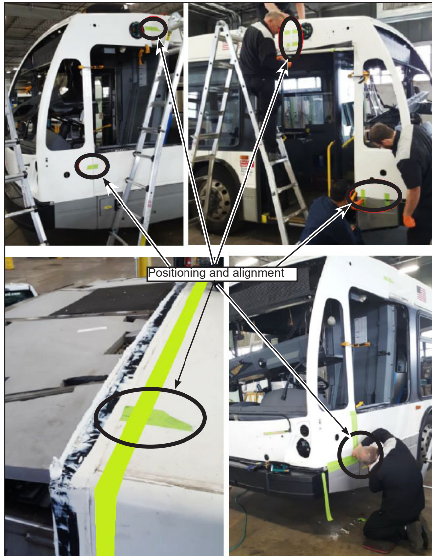
Figure 24 - Front Shell Dry Fit
