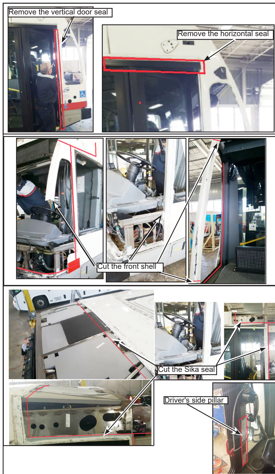
Figure 21 - Remove the Front Shell
