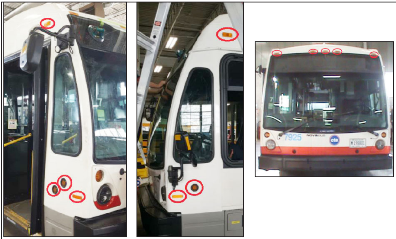
Figure 47 - Install Reflectors, Marker Lights and Signal Lights
