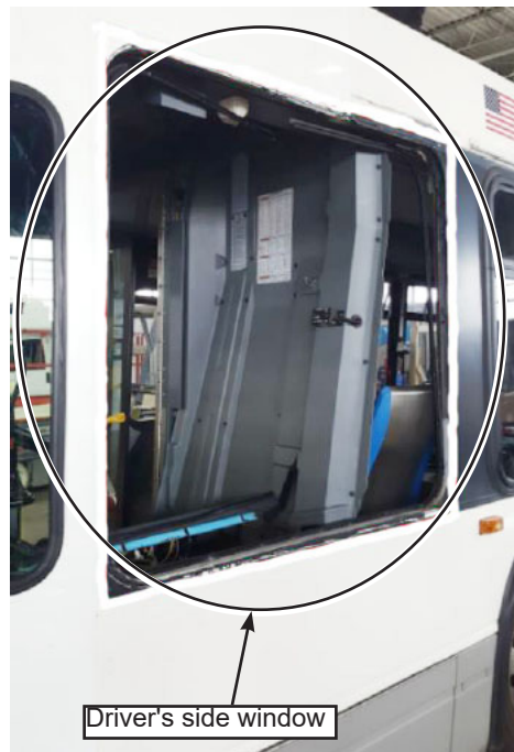
Figure 13 - Remove the Driver's side Window
