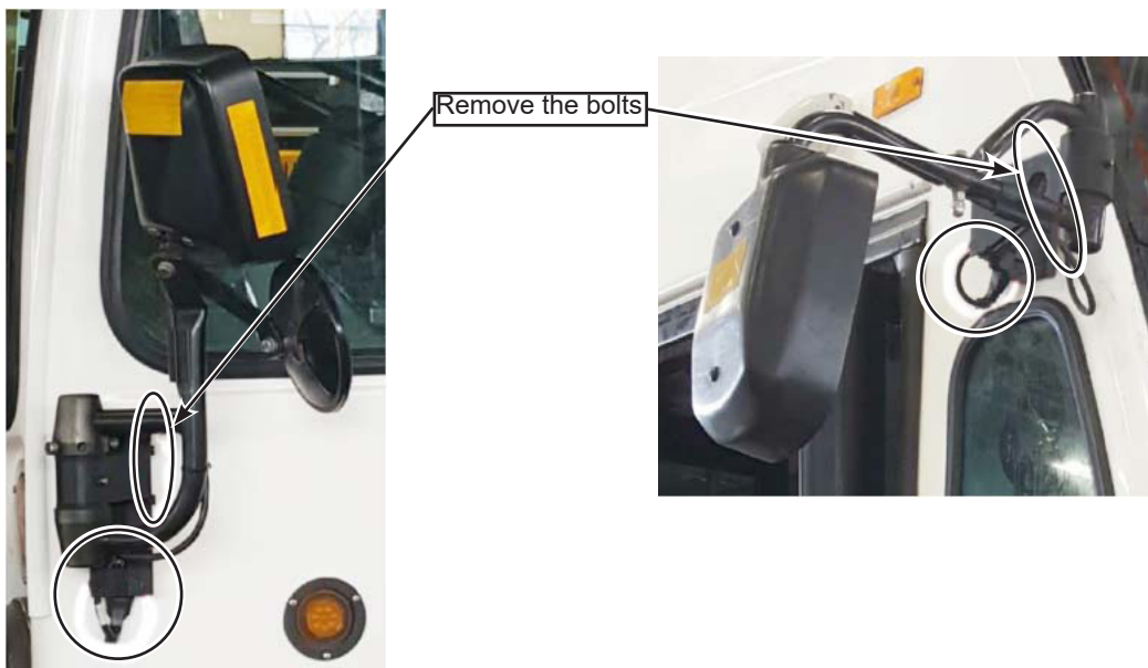
Figure 8 - Remove the Mirrors
