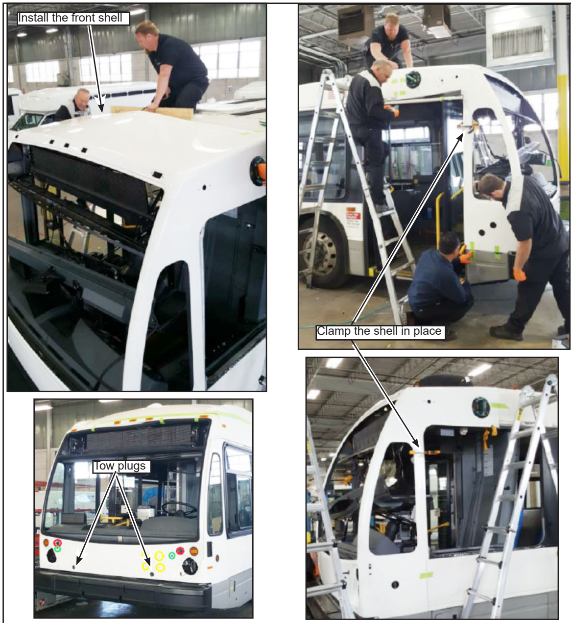
Figure 29 - Install the Front Shell
