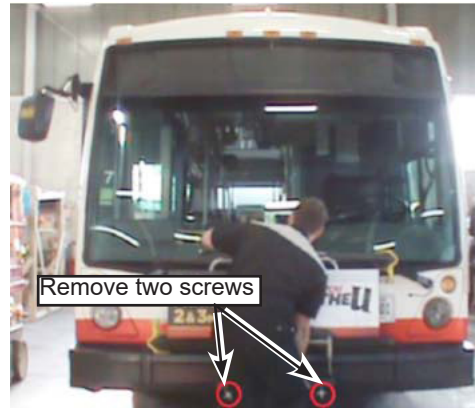
Figure 3 - Remove the Bike Rack
