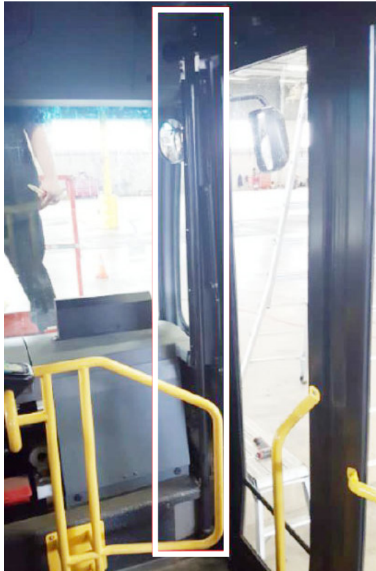
Figure 18 - Remove the Door Post Capping
