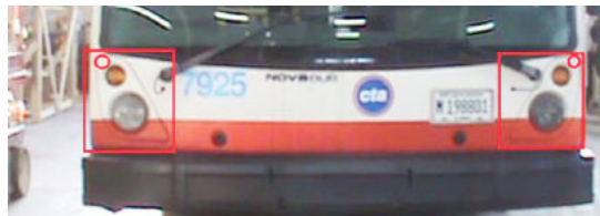
Figure 50 - Install the Turn Signals and Headlights
