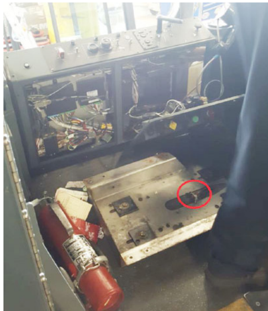
Figure 41 - Install the Driver's Seat
