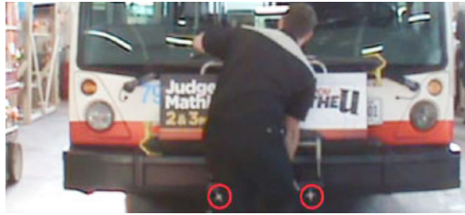
Figure 51 - Install the Bicycle Rack
