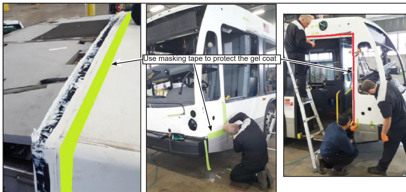
Figure 27 - Protect GelCoat with Masking Tape
