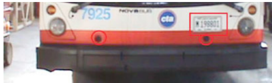
Figure 49 - Install the License Plate and Tow Plugs
