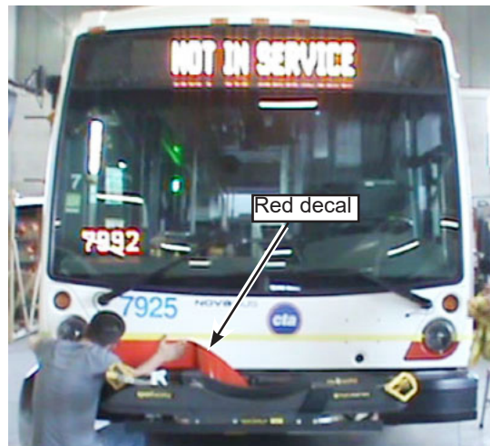
Figure 45 - Install the Red Decal
