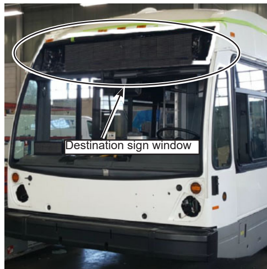
Figure 15 - Remove the Destination Sign Window
