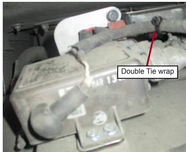
Figure 6 - Installation of Double Tie Wrap
