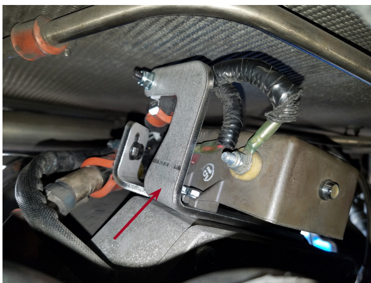
Figure 4 - Installation of Strain Relief Bracket on Regulator
