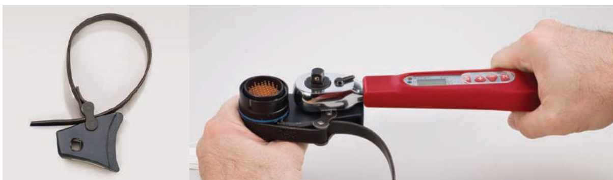
Figure 11 - Tightening the Connectors on Regulator
