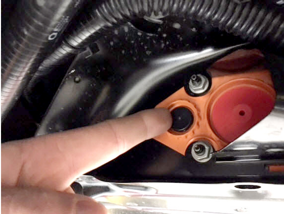
✓ Figure 1 (LH vent shroud with breather)
