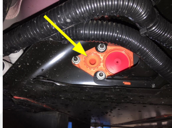
✗ Figure 2 (LH vent shroud without breather)
