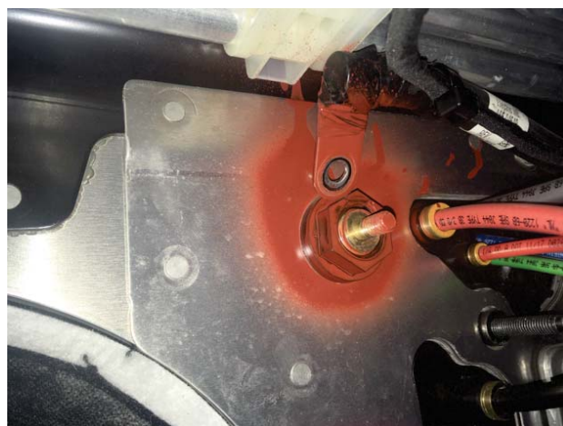
Fig. 7, GNDE Engine-Side Pass-Through Stud
