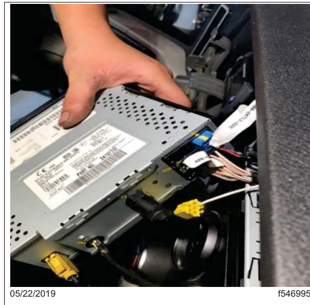
Fig. 3, Connectors on the Reverse Side of the Radio
