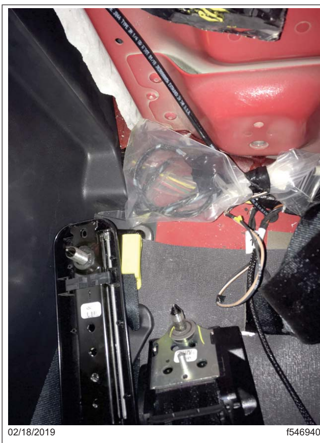
Fig. 12, Harness Secured Behind the Seat
