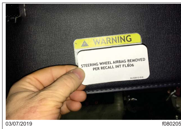
Fig. 15, Installing the Stickers on the Sun Visor
