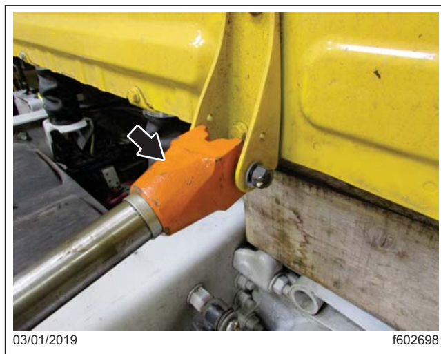
Fig. 4, Porta Power Applied to Shock Bracket Bolts
