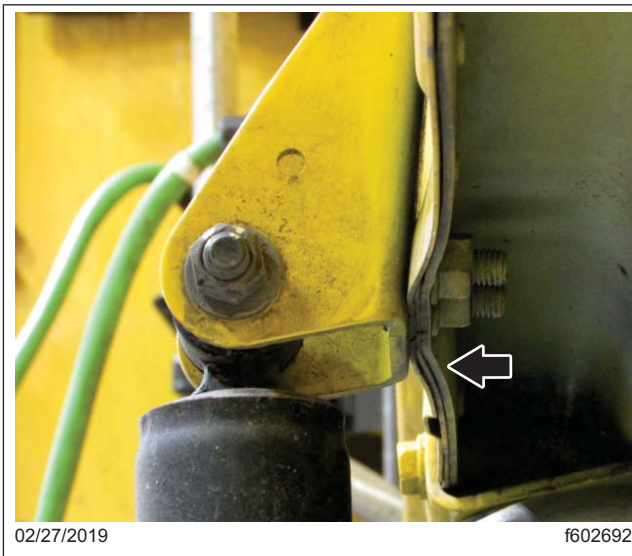
Fig. 1, Bending of Back Wall Centered on Shock Bracket
