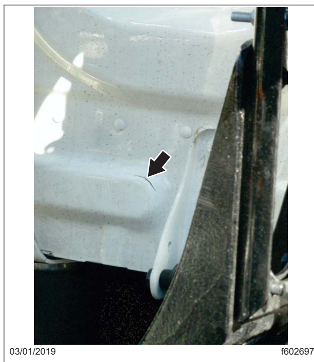
Fig. 3, Crack in Cab Back Wall
