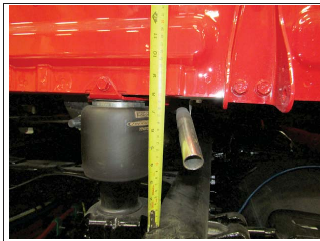
Fig. 7, Cab Raised Eight Inches Above the Frame
