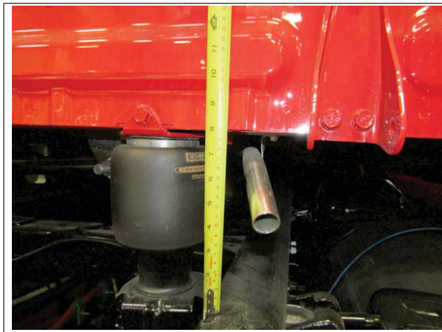
Fig. 7, Cab Raised Eight Inches Above the Frame
