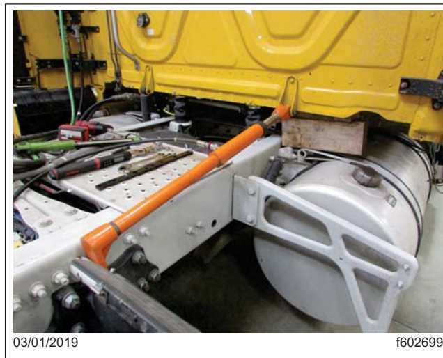
Fig. 5, Porta Power Set Up to Straighten Back Wall
