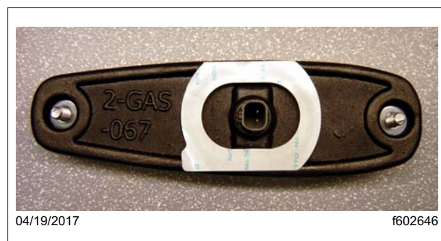
Fig. 1, Marker Light with Peel-and-Stick Adhesive Gasket
