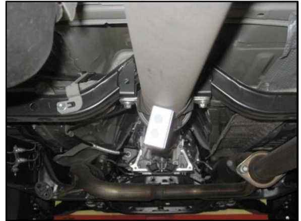
Figure 12. INCORRECT Placement of Digital Angle Gauge
