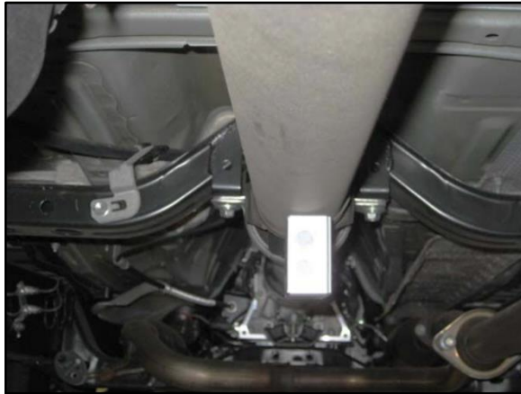
Figure 11. CORRECT Placement of Digital Angle Gauge
