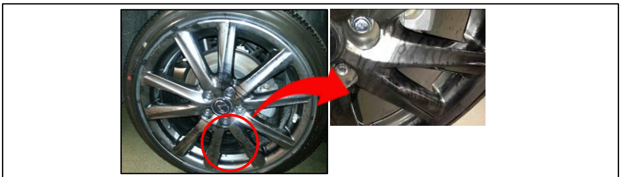
Figure 2. Additional Examples of Black Spotting (Not Brake Dust)
