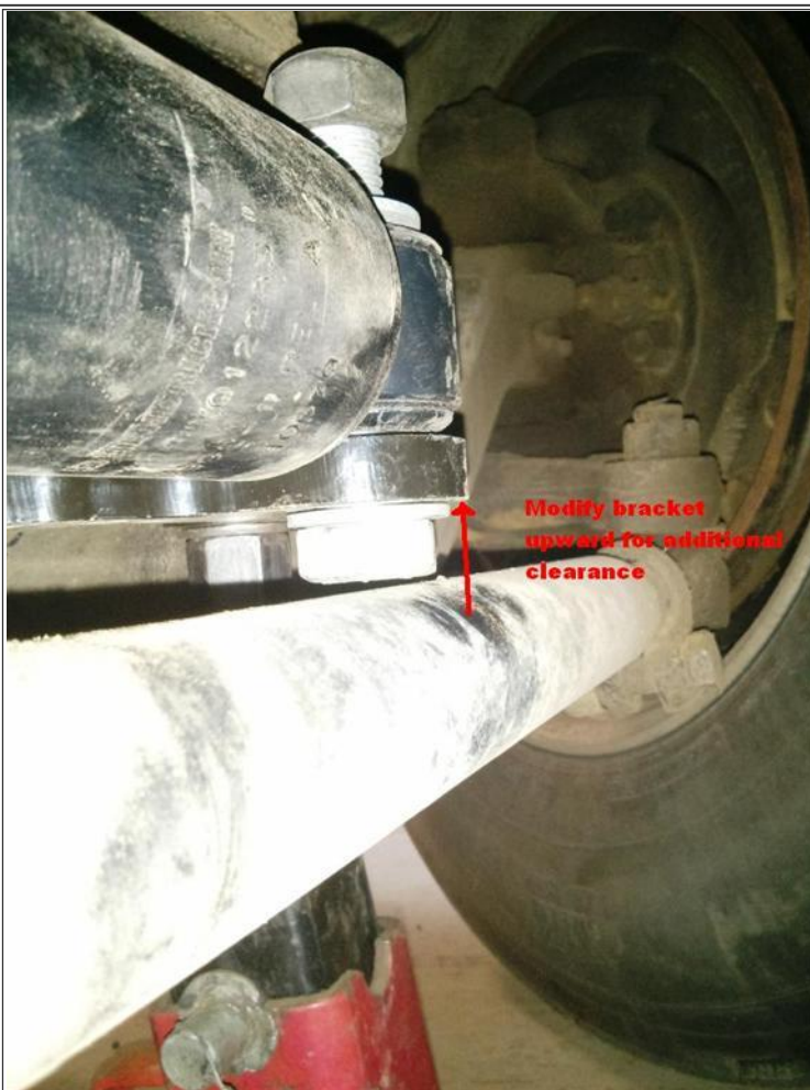
Figure 4: Tie rod tube to mount clearance
