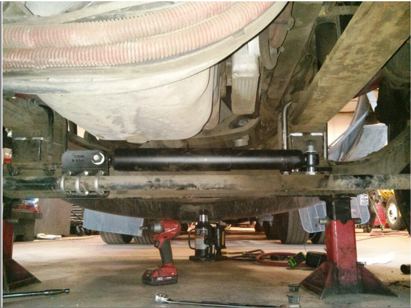
Figure 5: Assembled Steering Stabilizer
