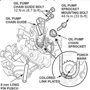
Apply new engine oil to the threads of the oil pump sprocket mounting bolt, then install it and torque it to **44** N·m (**33 Ib-ft**).
