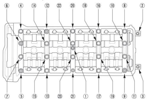
20. To prevent warpage, loosen the bolts in sequence 1/3 turn at a time, repeat the sequence until all the bolts are loosened. Remove the cylinder head bolts.
