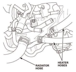
16. Remove the two bolts securing the connecting pipe. Disconnect the water bypass hose.
