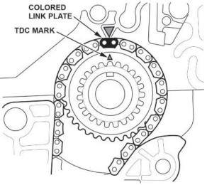
69. Set the oil pump sprocket on the oil pump chain with the punch mark aligned with the center of the colored link plates, then install the oil pump chain sprocket to the oil pump.
