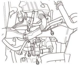
15. Disconnect the radiator hoses and the heater hoses. Disconnect the ATF warmer bypass hose (if equipped).
