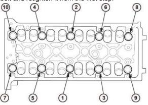
After torqueing, tighten all cylinder head bolts in two steps (90° per step) using the sequence shown above. If you are using a new cylinder head bolt, tighten the bolt an extra 90°.
