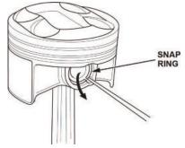
39. Put on gloves, heat the piston and the small end of the connecting rod to about 158°F (70°C), then remove the piston pin.
