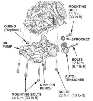
67. Align the dowel pin on the rear balancer shaft with the mark on the oil pump.
