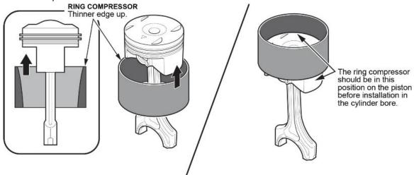
55. Set the ring compressor on the piston bore, then push the piston in with your hands.
