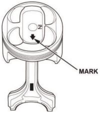
54. Set the piston in the ring compressor, and position the piston in the cylinder based on the rod/cap marks that you made in step 34.
