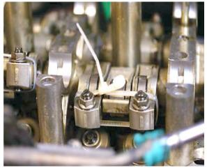
19. To prevent damage to the camshafts, loosen the bolts, in sequence, two turns at a time. Remove the camshaft holder bolts, Remove the rocker arm assembly and both cam shafts.
