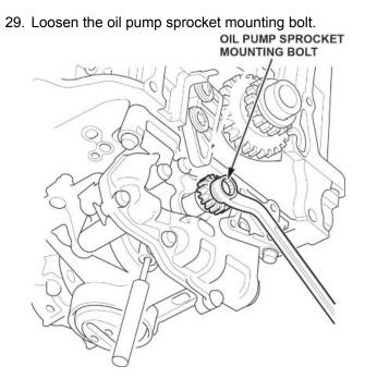
30. Remove the oil pump sprocket and the oil pump.
