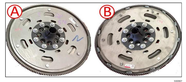
**Note:** Add medium strength thread locker to DSA flex plate clamp pinch bolt.
