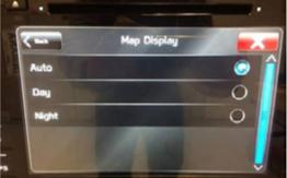
• If the instrument panel illumination control knob is set to MAX brightness (all the way up), the map display will not change regardless if "Auto" or "Night" mode is selected in Settings. Lower the illumination control knob as shown in the illustration and "Auto" or "Night" mode operation will be restored.
