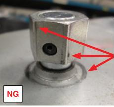
Witness marks on the hex portion and face plate of winch from using a deep-well socket and power tool.
