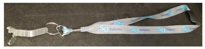
Simply drill a hole near the handle end of the tool and install an unused lanyard as shown above. The brighter color the better but, we liked the choice used here too!
